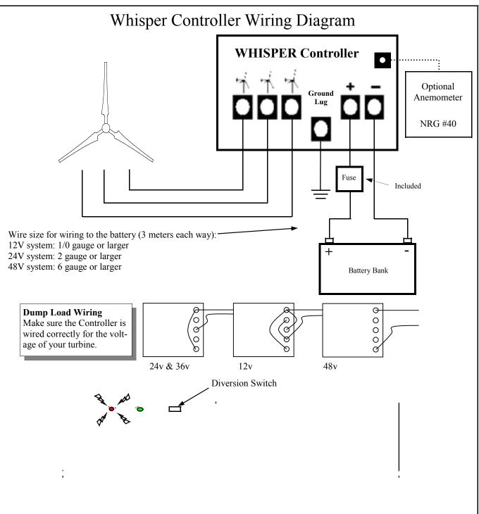
Once startup is successful and the red LED can be cycled by toggling the Diversion Switch, then set the switch to "Stop" (Red LED on) and connect the turbine wires to the controller (order of the turbine wires is not important). If the Red LED is on, the turbine will not spin as long as at least two of its wires are connected. For further operational information refer to Whisper Operation on page 16.
