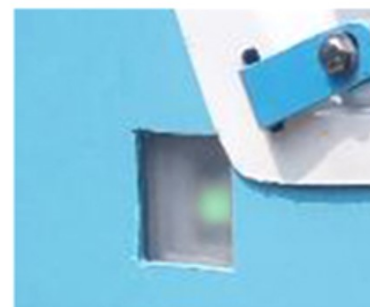
CHLORINE LEVEL INDICATOR
